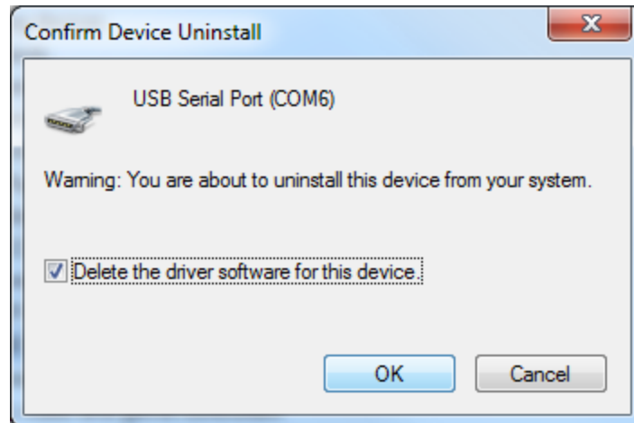
Figure 8: Uninstall comport to release assigned number
