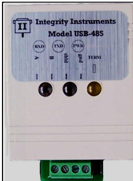
Figure 10: LED indicators (left to right) – RX | TX | PWR
